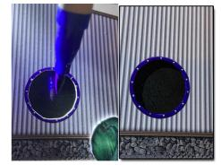
STEP 6-Touch up the inner edge surface with a small piece of sandpaper rounded file if needed. Next, with a blue watercolor marker to get rid of the white cardstock edge. This adds much greater realism. You are now ready to add the glass to the backside after step 7
