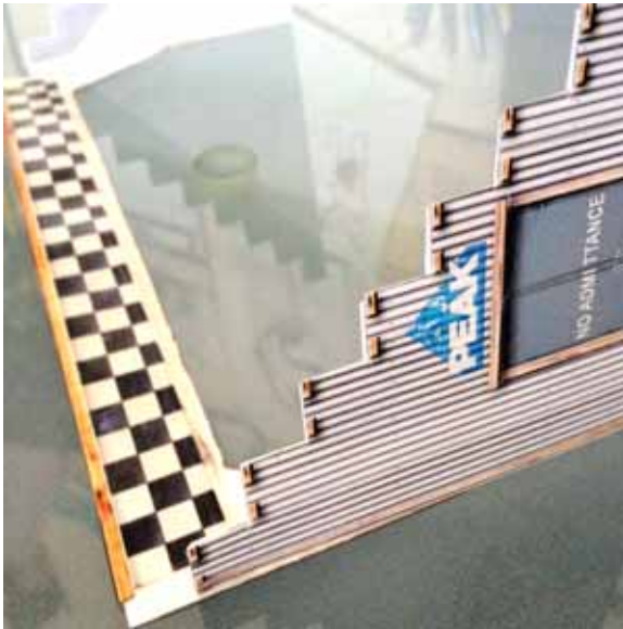
Figure 12 - Align and glue the supports and header.
